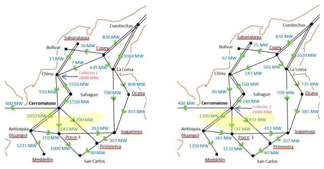
Figure 4-2 Network power flow based on the Collector 2 interconnection location in 2032 Max Dem Max Gen study case (Left: at Chinu, Right: at Cerromatoso)
