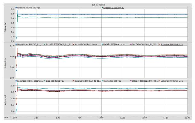
Figure 3-10 Selected 500 kV bus voltages (Contingency 1, 2032 Max Dem Max Gen—Alternative 4)
