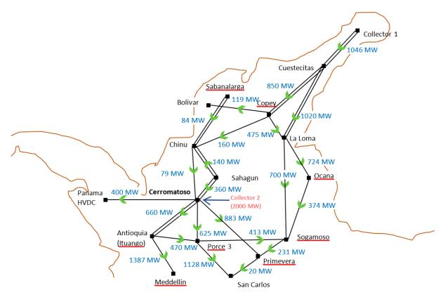
Figure 3-2 Active power flow on selected 500 kV transmission corridors - 2028 Max Dem Max Gen
