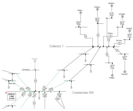
Figure 3-5 AC System strength at Cuestecitas—2028 Min Dem Min Gen
