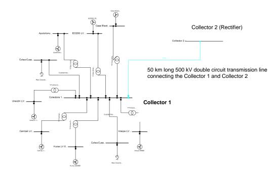
Figure 3-12 LCC HVDC transmission system rectifier at the Collector 2
