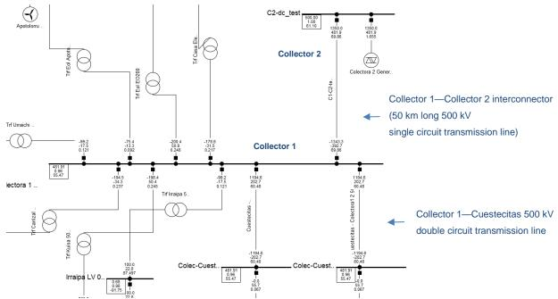
Figure 4-5 Collector 2 to Collector 1 Power flow during a HVDC pole outage (2032 Max Dem Max Gen)
