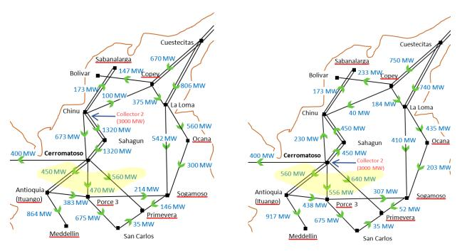
Figure 4-1 Network power flow based on the Collector 2 interconnection location in 2032 *Min Dem Min Gen* study case (Left: at Chinu, right: at Cerromatoso)
