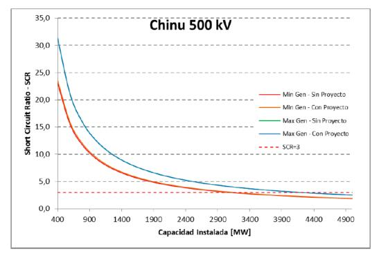
Figure 2-3 SCR relationship to connect generation in Chinú [1]
