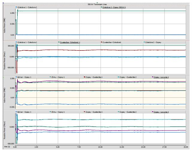
Figure 3-9 Active power flow on selected 500 kV transmission lines (Contingency 1, 2032 Max Dem Max Gen—Alternative 4)
