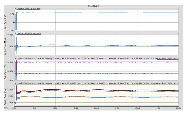
Figure 3-11 Renewable generation at Collector 2 and Collector 1 (Contingency 1, 2032 Max Dem Max Gen—Alternative 4)
