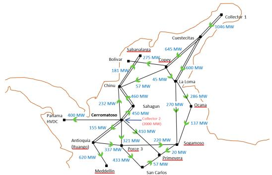
Figure 3-1 Active power flow on selected 500 kV transmission corridors - 2028 Min Dem Min Gen
