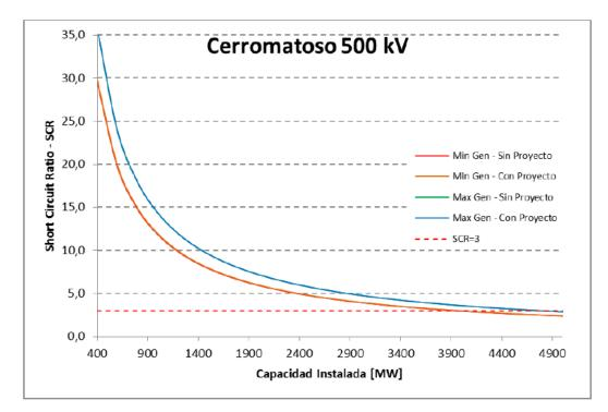
Figure 2-4 SCR relationship to connect generation in Cerromatoso [1]
