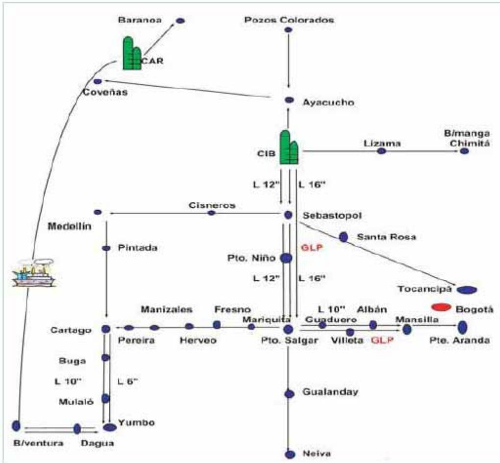
There is a fuel oil pipeline that transports surplus fuel oil from the Barrancabermeja refinery for the foreign markets. This pipeline joins the Coveñas port with the mentioned refinery and has two intermediate stations: One at Ayacucho and the other at El Retiro. All along the pipeline grid there are intermediate stations where product is stored in warehouses in case of contingencies, owned by a fuel wholesale distributors of petroleum byproducts.
